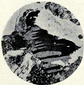
5.—Biotite. Ord. L. Showing partial alteration to chlorite.
